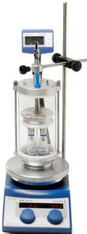
**The DrySyn Spiral Evaporator from Asynt allows users to vacuum down up to four different samples at a time, streamlining work-up procedures for multiple reactions**
