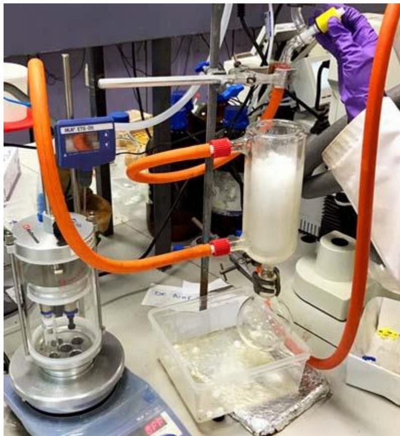
**The DrySyn Spiral Evaporator from Asynt allows users to vacuum down up to four different samples at a time, streamlining work-up procedures for multiple reactions**
